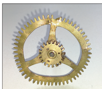
Figures 6 and 7. The clock as received in 2017 had extensive damage, for instance (left) by application of excessive force, and (right) a tooth lost by apparently having been cut too deeply. The early remedy: a replacement tooth from the tip of an added crossing..
