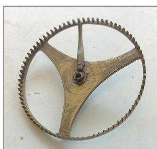
Figures 6 and 7. The clock as received in 2017 had extensive damage, for instance (left) by application of excessive force, and (right) a tooth lost by apparently having been cut too deeply. The early remedy: a replacement tooth from the tip of an added crossing..
